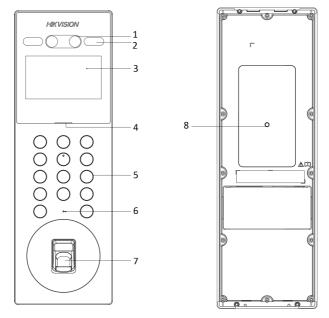
Figure 1-2 Appearance of Door Station with Fingerprint Module Table 1-2 Description
