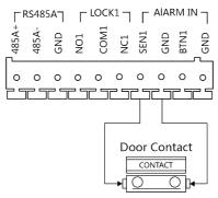
Figure 2-4 Door Contact Wiring
