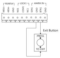
Figure 2-3 Exit Button Wiring
