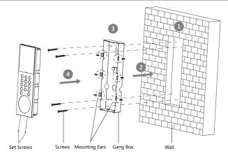
Figure 3-2 Flush Mounting with Gang Box
